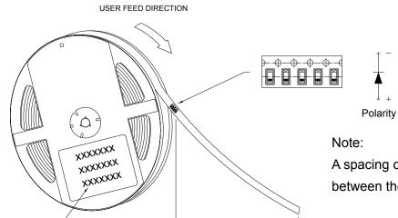
A spacing of approximately 160mm between the front edge of tape
